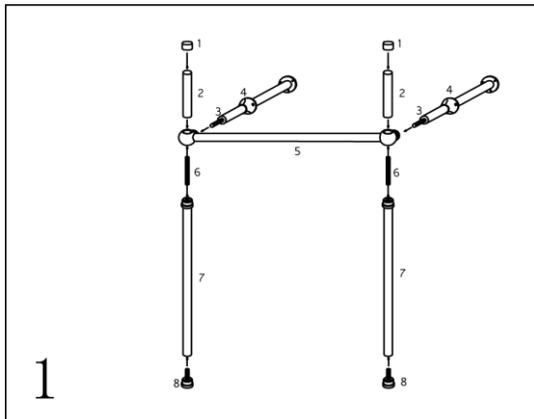
1. Place metal base stand assembled in accordance with the drawings shown. Ensure that you have all parts necessary. Then assemble each part per diagram Do not lock wall support bar SHCS decorative cover.
