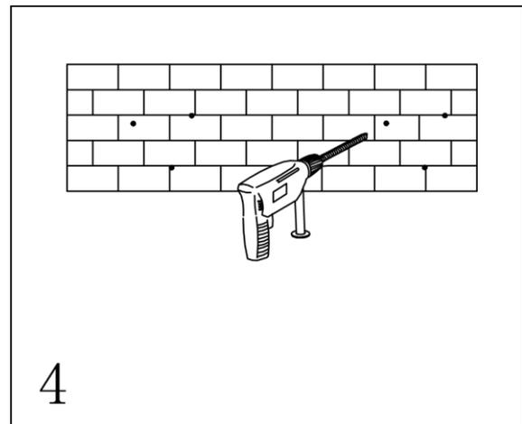
Step 4. Take the drill and drill a 6x25mm hole (the size of the plastic anchor). Measure the length of the expansion pipe , For professional workers ( Or do it yourself ) Use the impact drill (drill specifications M6) Good point taken in the third step drill , The depth of the hole is determined based on the measurement results After taping the plastic expansion pipe (anchor) , Neither prominent expansion pipe wall , Nor sunken into the wall is appropriate
