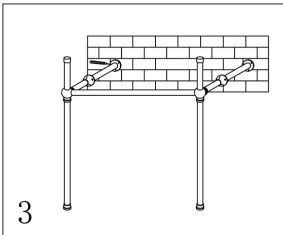
Step 3. Please metal base stand assembled in accordance with the drawings shown , Take the pencil and mark the designated where you will drill the holes for the metal base stand. Once you have you marked the specific area. Remove the stand and set it aside for now.
