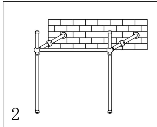
2. The assembled ready to install metal base stand is placed in the wall( Please give specific installation location for the drainage hole position to insure your plumbing is in the correct place.)
